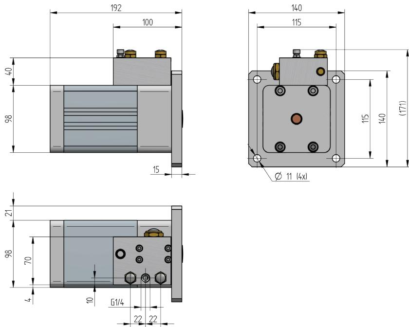
The KFZ-080 pneumatic impactor is converting pneumatic energy from compressed air into mechanical energy. It generates impulses comparable to a hitting hammer for knocking stubborn residues from walls, pipes and containers.
